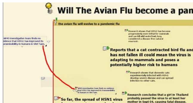
Figure 14: An Assertion with Evidence Gates. As the analyst drags evidence through the left refuting gate of an assertion, the gate flashes red, the evidence is tagged with a minus sign and the red visual indicator on top of the assertion grows. A corresponding supporting gate, on the right side, flashes green, adds a plus sign and updates the green bar of the assertion score when used.
